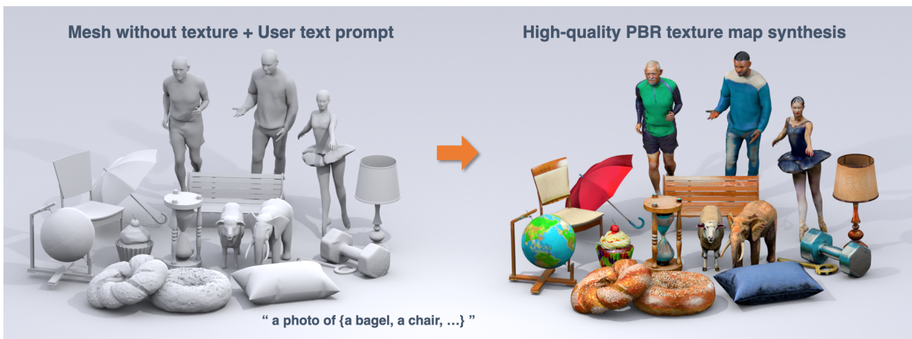
Figure 1. Paint-it . Given an untextured 3D mesh and the text description describing the desired appearance of the 3D mesh, Paint-it automatically synthesizes high-fidelity physically-based rendering (PBR) texture maps by neural re-parameterized texture map optimization.
